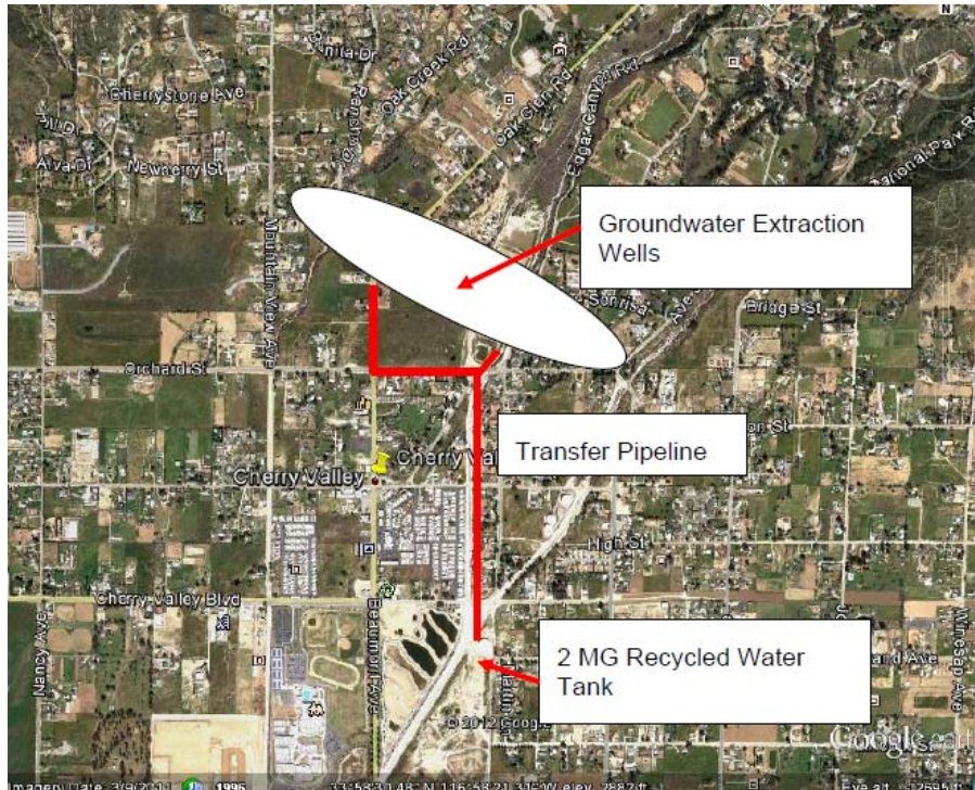
Figure 4-16 Groundwater Extraction Project (Pollution Control Project)
