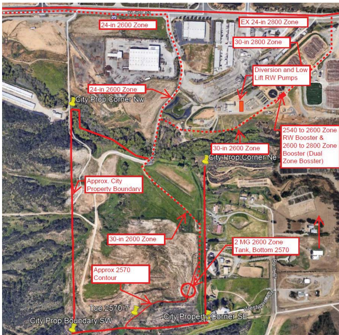
Figure 4 Tentative Plan for Non-potable Water Facilities at City of Beaumont Wastewater Treatment Plant
