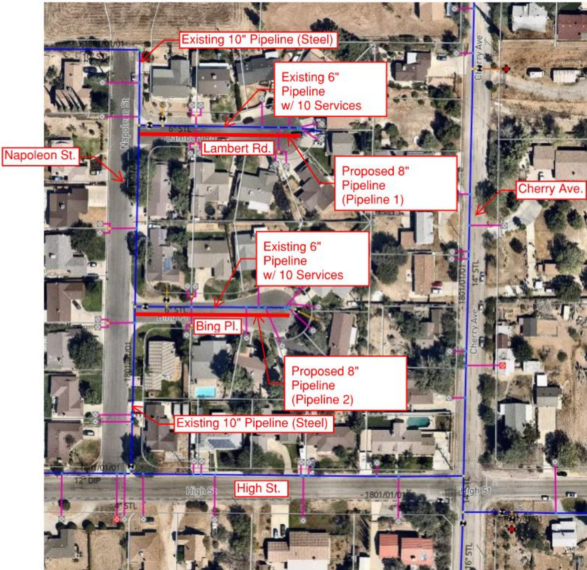
Figure 3 Pipelines 1 & 2 (P-3040-0023 & P-3040-0024) Site Map
